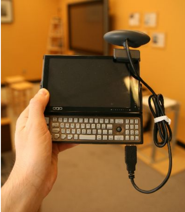
Figure 2. The OQO UMPC with an attached webcam can be held in one hand.
