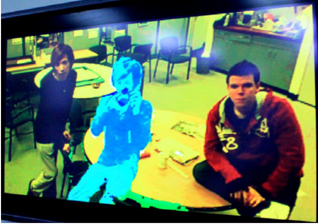
Fig. 2. The Looking Glass projects a user into the captured scene as a ghost-like blue figure, while the captured scene is tinted yellow for an 'old sepia photo' effect
