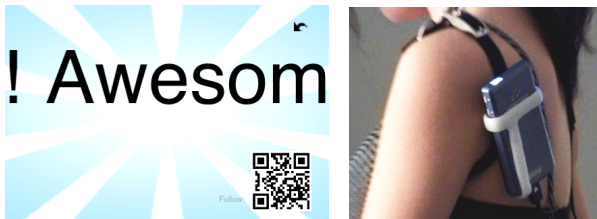
Figure 1: A new message posted on the halo with a QR marker at the bottom right corner (right); Wearing the Tweeting Halo (left).
