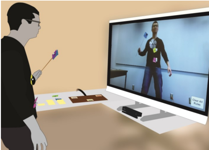
Figure 1: Bod-IDE with a designer standing in front of the 'mirror' display with some tags fastened to their body and a prop.
