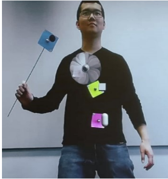
Figure 2: The mirror display (zoomed for clarity) with a designer wearing multiple tags and an augmented prop. Virtual components are rendered in real-time.
