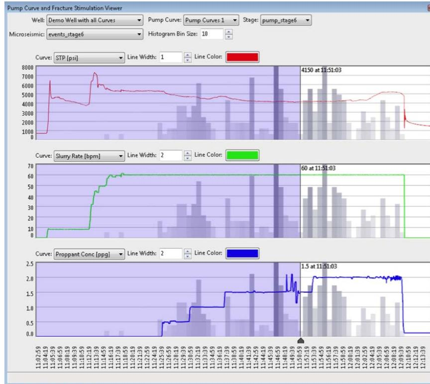
Figure 3.1: Example of the microseismic engineering (pumping) curves [6]
