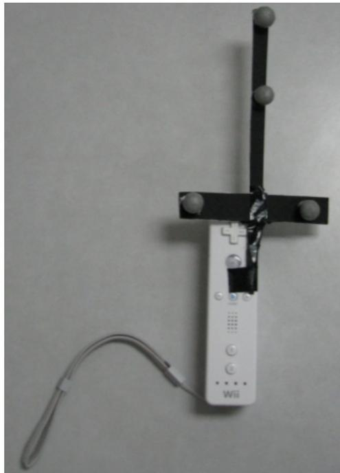
Figure 4.5: The Wii controller (with attached markers) used in our prototype for pointing and interaction.
