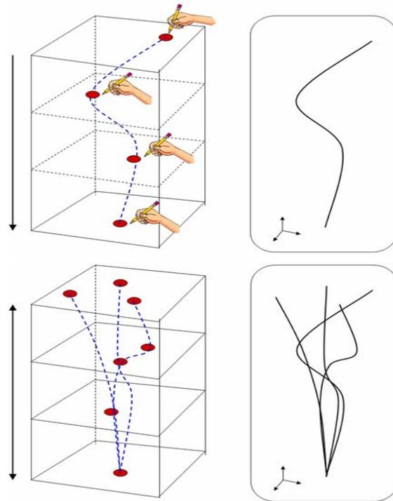
Figure 4. Input of 3D branch line structures with the 3D Tractus.
