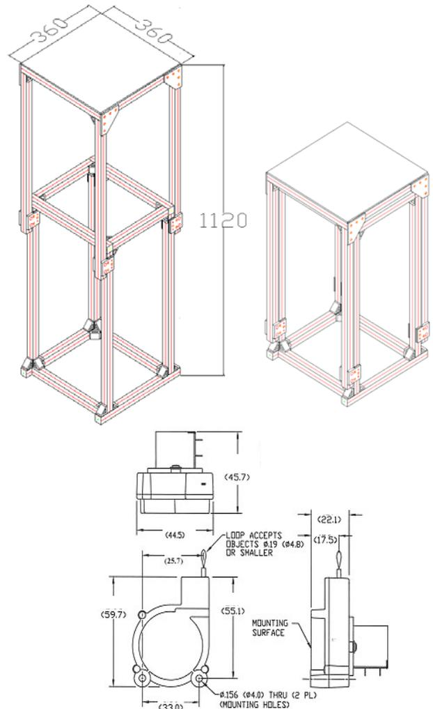
**Figure 3. The 3D Tractus prototype (top), Sensing height with a string pot (bottom). All dimensions are in millimeters.**
