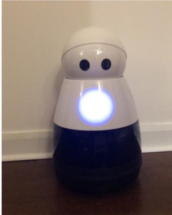
**Figure 3:** Kuri is a small social robot. It's interaction involves autonomous or app controlled movement, expressive eyes, babbling sounds, and a heart light that produces different colours.
