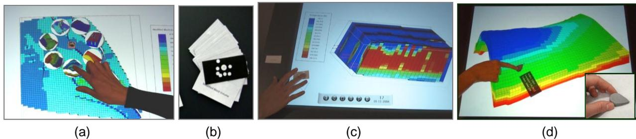
Figure 3: (a) Reservoir model selection menu, and (b) property cards, activated when (c) placed on the screen. The time step navigator is depicted, selected on step 17 (01-11-2004); (d) the cell probe displaying cell-specific info.
