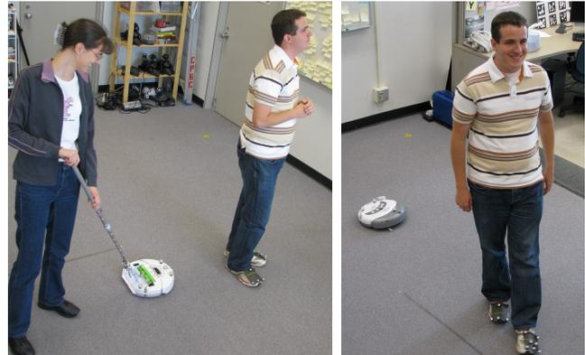
**Figure 1 – Style by demonstration: a person (left) shows the robot the style of how to interact with a person (e.g., follow politely), and (right) the robot mimics the demonstration to follow politely.**
