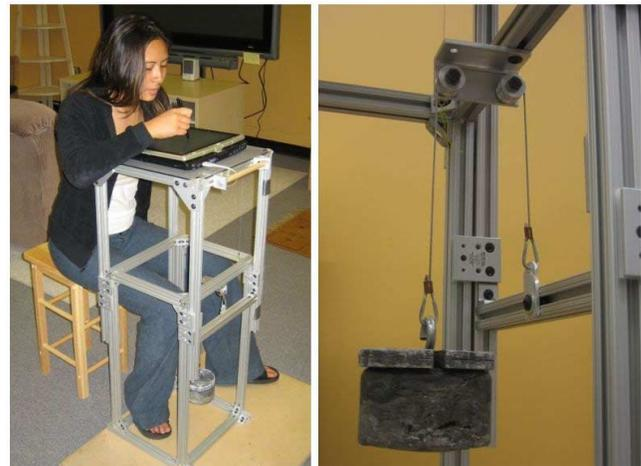
**Figure 6: The 3D Tractus frame and counter-weight.**
