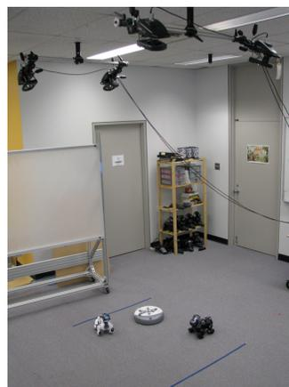
(b) The robot workspace with Vicon cameras and robots.
