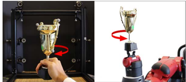
Figure 1: ReMa – Remote Manipulator: While the end position is the same, the robot's movement trajectory to the goal position (right) does not match the human motion (left) due to the "wrist" joint limitation of the robot
