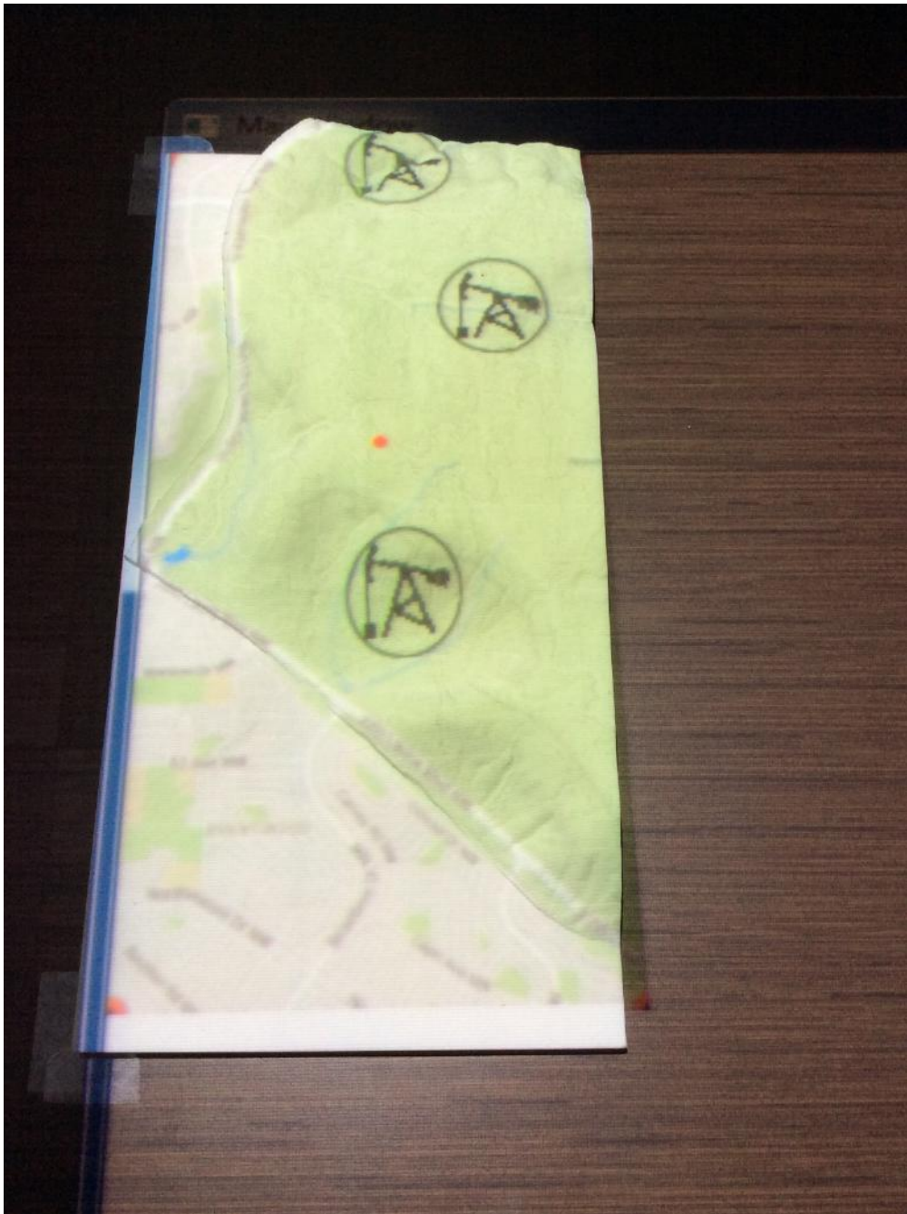
Figure 6.2: Projection Based Augmented Reality overlays content on to the 3D printout
