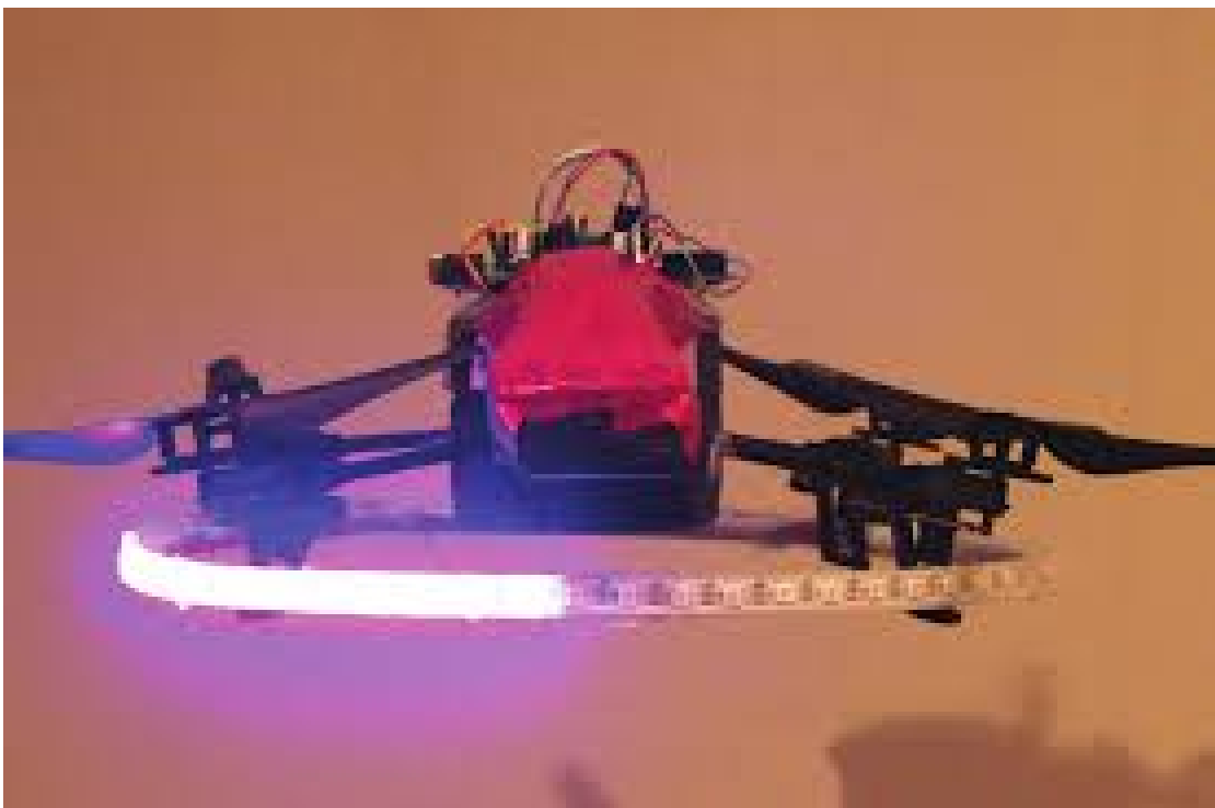
Figure 2.17: [szafir et al.2015] explored the design of visual signalling mechanisms for flying robots to support the expression of robot intent and increase usability in collocated interactions.
