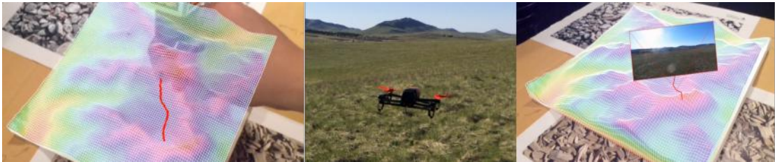
Figure 5.3: Flying Frustum ; (left) the operator draws a path using a pen on the augmented 3D printout of the terrain; (middle) the UAV, a quadrotor in the current prototype, flies along the path in the field; (right) live video footage streaming from the UAV is displayed as a view frustum situated at the correct location on the 3D printout, using augmented reality
