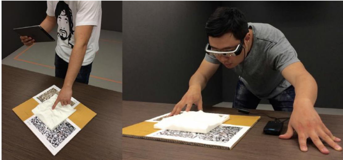
Figure 5.6: ( Flying Frustums augmented reality devices including (left) handheld screen and (right) see-through headset
