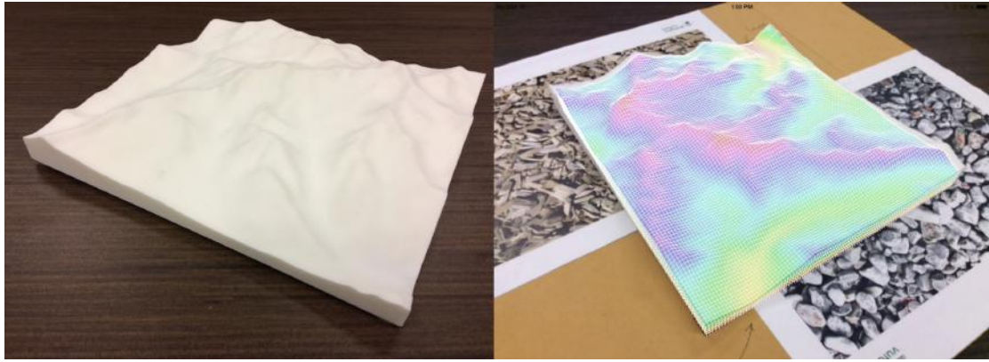
Figure 5.5: (left) using a 3D printout model as a physical representation to the topographical terrain; (right) augmented reality visualization is superimposed onto the model
