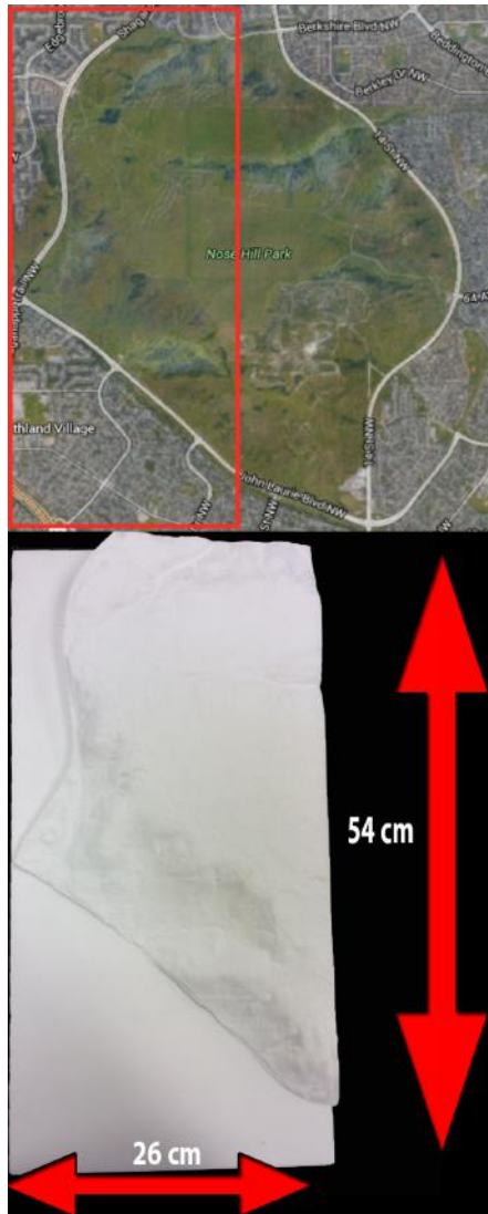
Figure 7.2: (top) Google map image of the wilderness park near out university. The red rectangle is the area which we 3D printed and (bottom) the 3D prinout of the area marked in the google map image.
