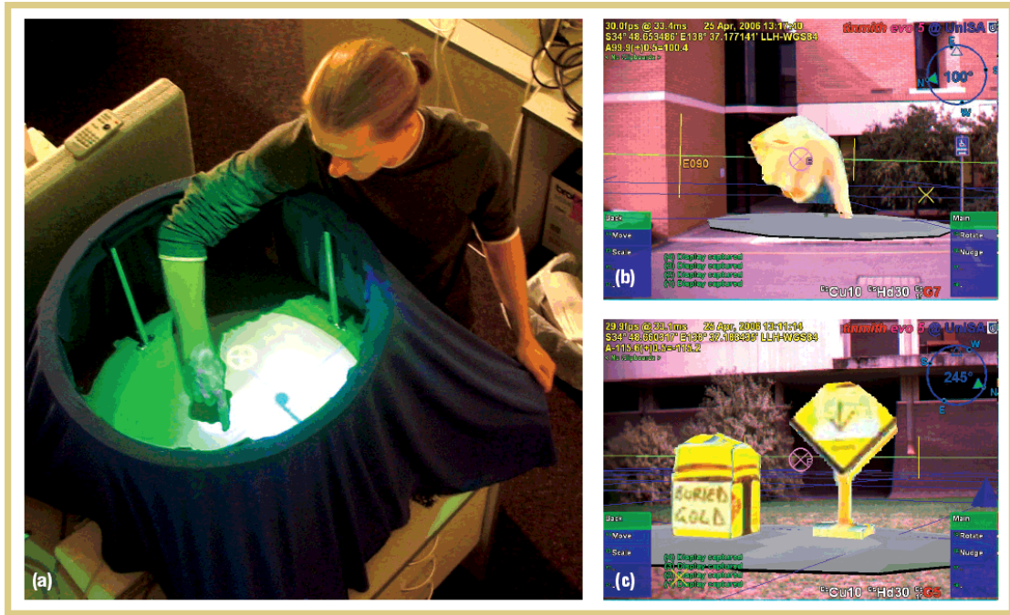
Figure 2.9: God-Like Interactions by [Stafford et al., 2006]. (a) indoor user pointing at a location on the table-top surface, which contains the representation of the outdoor world. (b) Outdoor AR view showing the indoor user’s hand appearing from the sky and pointing toward a location in the distance.(c) Physical objects used as props to convey extra meaningful information about the environment.
