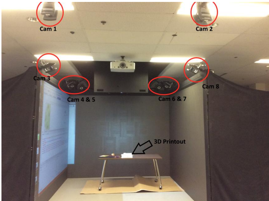
Figure 7.5: Our projection-based augmented reality setup. A Vicon system with 8 cameras is used for tracking the stylus.
