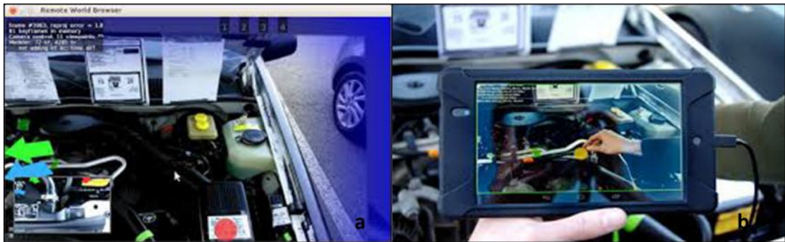
Figure 2.10: World-Stabilized annotations for live mobile remote collaboration [Gauglitz et al., 2014]. (a) Screenshot of the remote helper interface. (b) Screenshot of the local user with live annotations made by the remote user.
